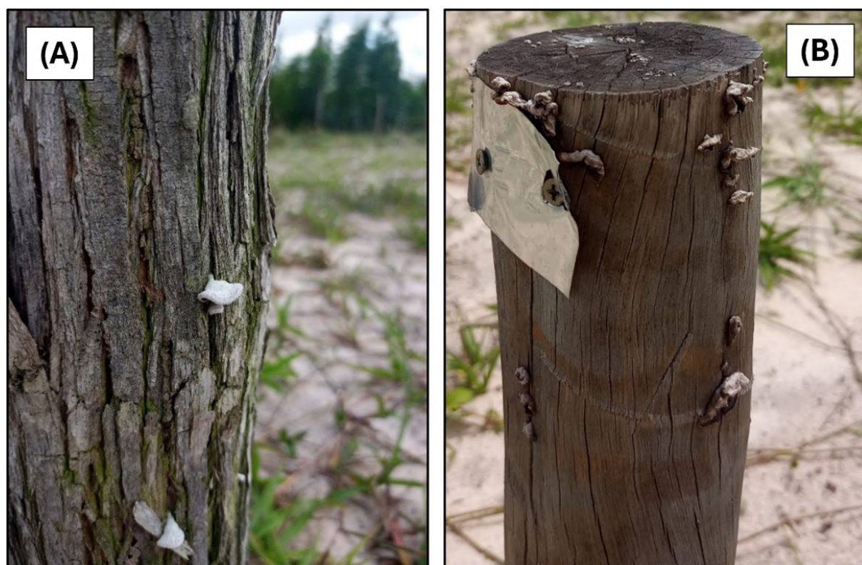
Figure 4. Presence of fungi (mushrooms) in the round wood pieces of M. caesalpinii (A) and treated Eucalyptus (B) after two years of exposure in the field
